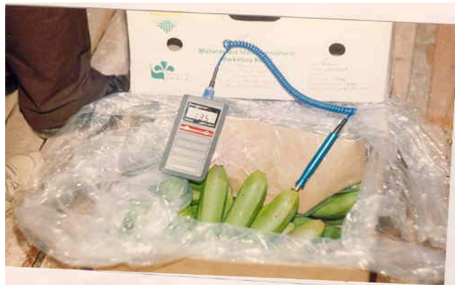
TEMPERATURE MEASUREMENT ON TRANSFER OF BOXES TO COLD STORAGE
