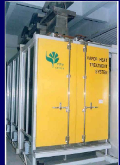
Vapour heat treatment system
